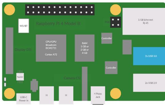
**Fig. 6.** Raspberry Pi Architecture.
